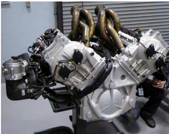
Porsche 918 engine out of one of the prototype cars used for training dealership mechanics on the 918
