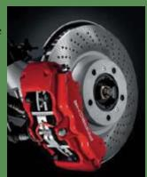
brake fluid, I must touch upon the required 2 year maintenance of flushing ones brake system. Brake fluid is hygroscopic. It readily absorbs moisture, and the boiling point is thus affected. Porsche brake fluid has a wet boiling point of 356°F. Not flushing the fluid can severely limit a track day. In fact, PCA events require a yearly service interval on brake fluid instead of the Porsche required 2 year interval.
